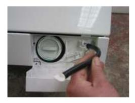
If a pipe like this is fitted to your machine, pull the stop from the end of the pipe, and drain the water that is left in the machine into a suitable container. This will save you getting water on your floor, when you remove the filter. Even if the machine has pumped the water out, there will always be some water left in the sump. Always refer to manufacturer's handbook.
