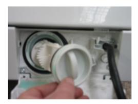
This is an example of a typical filter being removed. Clear out and refit.
